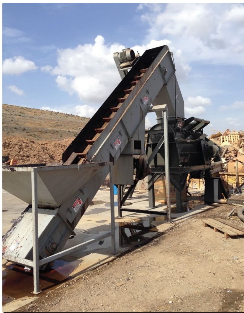
Colony Energy is using a Scott's Turbo Separator to depackage and blend incoming food waste feedstocks. Photo courtesy of Colony Energy Partners
